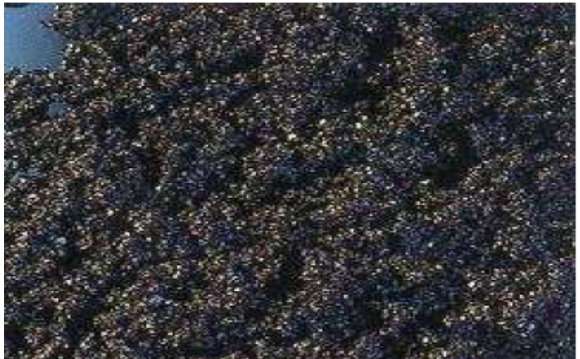
Granular ferric hydroxide arsenic removal media
