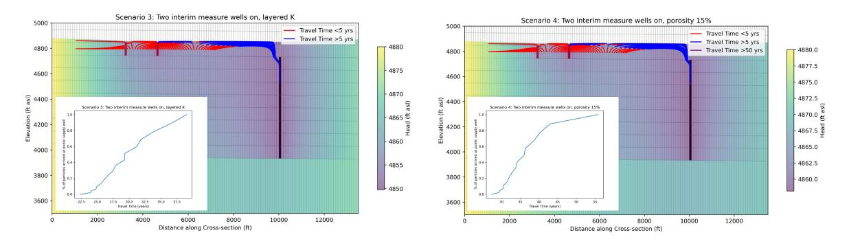
> Variations in model parameters speed up or slow down time to breakthrough, highlighting the importance of input parameters
