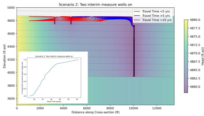
2 extraction wells off, new pumping rate at remaining extraction wells
